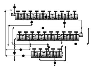
Fig. 1. Flotation circuits sampling points
