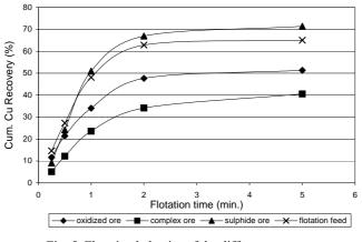
Fig. 5. Flotation behavior of the different ore types
