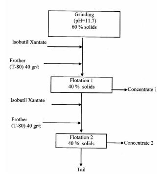
Fig. 4. Laboratory flotation test procedure
